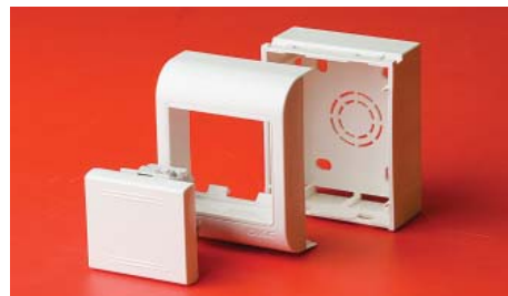
1. Boxes of PDD type for wiring devices "Viva", "Brava", and with dimensions of 45x45 mm. Sockets in these boxes are installed by latching (without carriers and frames). The boxes have pre-perforation for all the standard sizes of TMC series miniducts on 4 sides
