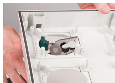
Elements with pre-perforation shall be removed for 32 A socket installation
